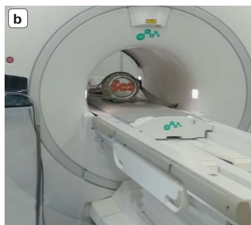
Fig. 2. Scheme of the experiment: a – installation of ready-made test tubes in a phantom; b – MRI examination of a phantom with a GEM Flex Body radiofrequency coil.
